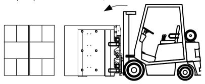
1-2) Align the bottom of the attachment to bottom of the load.
