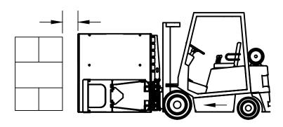
1-3) Align the bottom of the attachment to bottom of the load.
