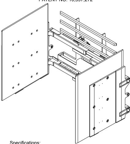
Specifications: Mounting: Class II Side Shifting: Internal Side Shifting Capacity: 2000 lbs at 24" Pad Size: 60" High x 48" Long Range: 22.4" - 94.4" Frame: 59" Wide
