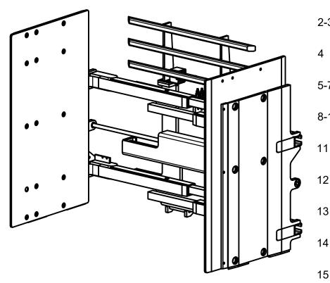
Specifications: Mounting: Class II Side Shifting: Non Side Shifting Capacity: 2000 lbs at 18" Pad Size: 55" High x 34" Long Range: 21.8" - 83.0" Frame: 48" Wide
