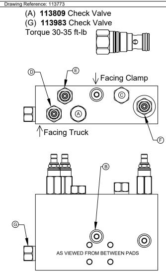
NOTE: Lubricate threads & seals prior to assembly.
