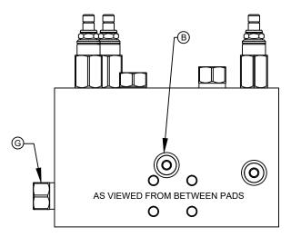
NOTE: Lubricate threads & seals prior to assembly.
