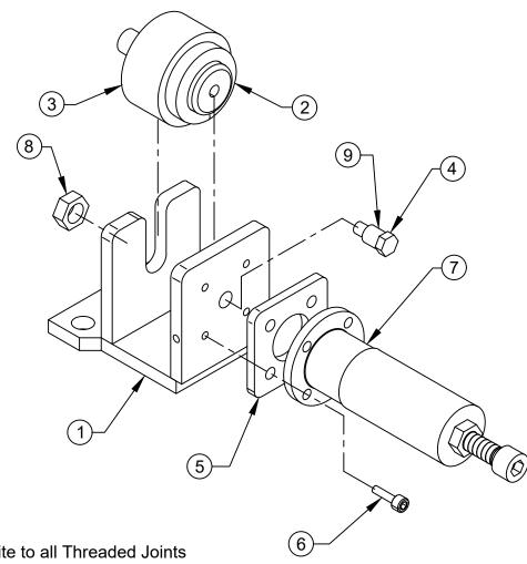
Note: Apply Loctite to all Threaded Joints
