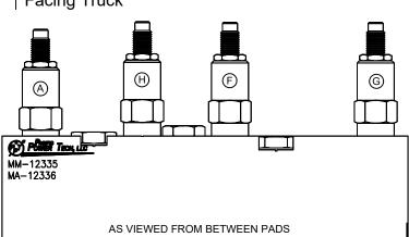
**NOTE:** Lubricate threads & seals prior to assembly.
