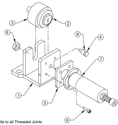
Note: Apply Loctite to all Threaded Joints
