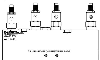
**NOTE:** Lubricate threads & seals prior to assembly.
