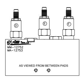
(C) **112887** Flow Divider Torque 10-12 ft-lb Seal Kit 104711
