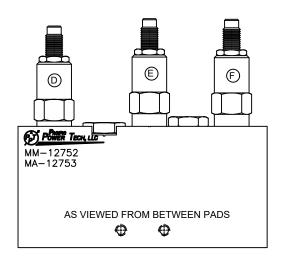
(C) 112887 Flow Divider Torque 10-12 ft-lb Seal Kit 104711
