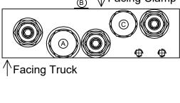
(C) **112887** Flow Divider Torque 10-12 ft-lb Seal Kit 104711
