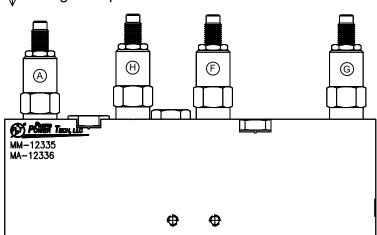
NOTE: Lubricate threads & seals prior to assembly.
